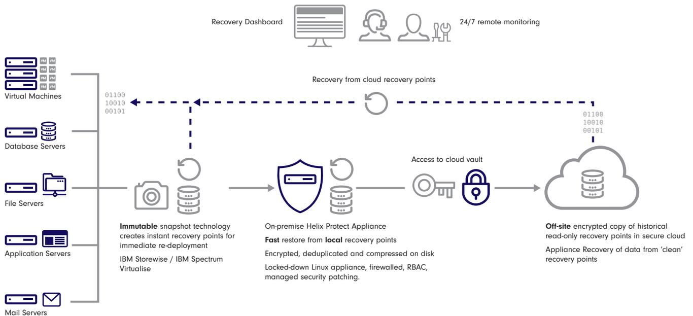
Three tier architecture, designed to provide fast recoveries with insurance against data loss using data protection technologies.
