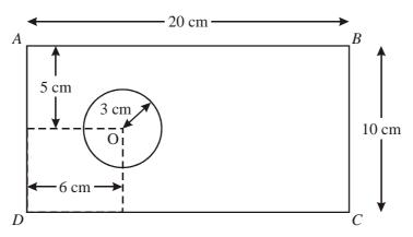
This diagram shows a metal plate that is made by removing a circle of centre O and radius 3 cm from a uniform rectangular lamina ABCD, where AB = 20 cm and BC = 10 cm. The point O is 5 cm from both AB and CD and is 6 cm from AD.
