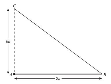
A uniform rod AB, of length 8a and weight W, is free to rotate in a vertical plane about a smooth pivot at A. One end of a light inextensible string is attached to B. The other end is attached to point C which is vertically above A, with AC = 6a. The rod is in equilibrium with AB horizontal, as shown in the diagram.
