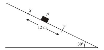
A small package P is modelled as a particle of mass 0.6 kg. The package slides down a rough plane from a point S to a point T, where ST = 12 m. The plane is inclined at an angle of  $30^{\circ}$  to the horizontal and ST is a line of greatest slope of the plane, as shown in the diagram. The speed of P at S is S is S in S and the speed of S and the speed of S is S in S
