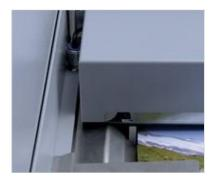
Two delivery sections The delivery side consists of two different output levels. For creasing and folding, the upper delivery belt is used, for creasing only the lower reception tray.
