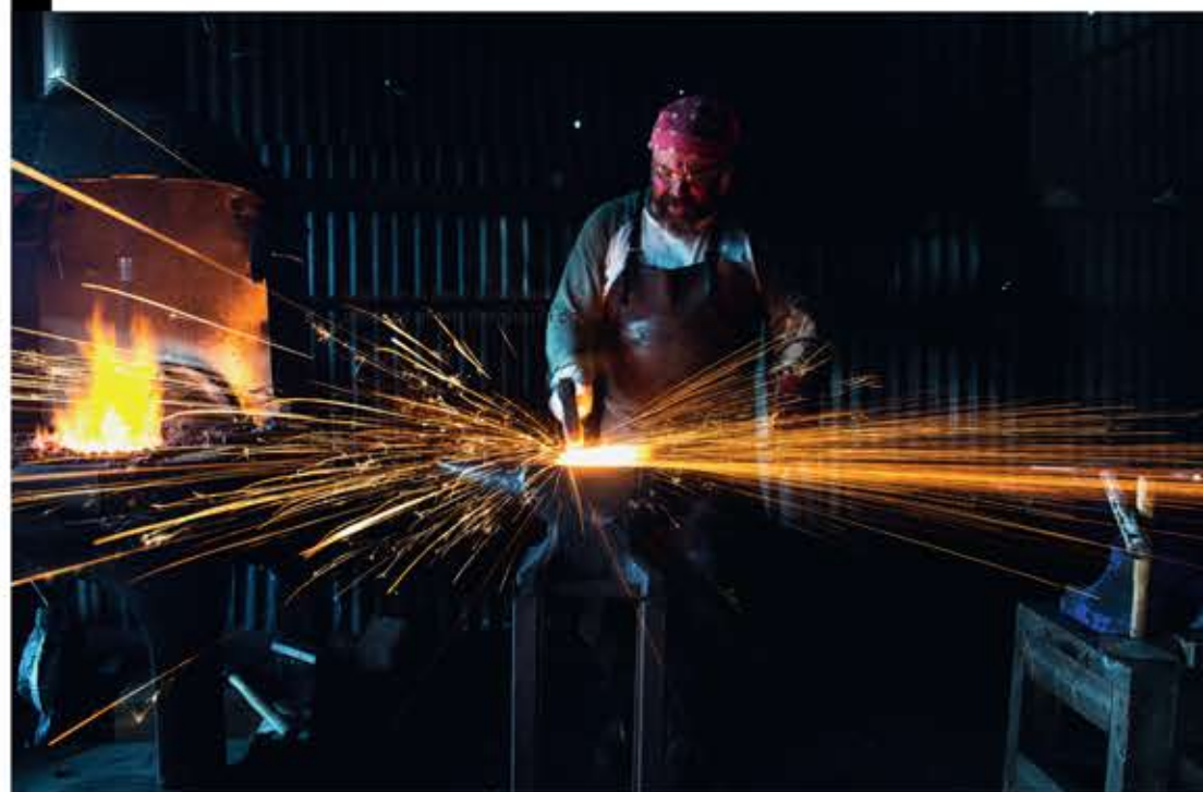
Left: hammering and folding layers of Damascus steel
