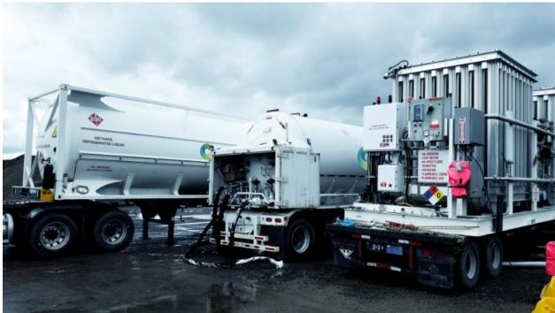
CLEANCOR's mobile equipment packages are designed to let an asphalt plant temporarily operate on LNG while the plant is being permanently transitioned to LNG as its fuel source.
