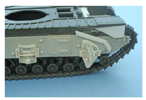
The attachment brackets in detail with changes to the mudguard profile and mud chute
