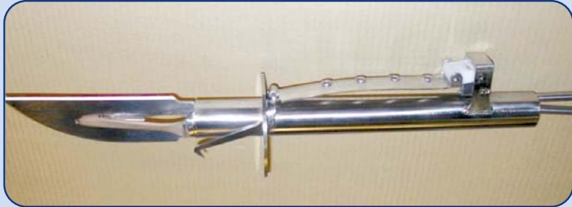
Anticoagulant must be added at the collection point, at the knife blade itself (in-case of using a hollow-knife), otherwise the blood coagulates in the knife and in any pipe or pump and blocks everything. Coagulation inside equipment makes it “impossible” to clean, at least during normal production. The longer the time allowed for bleeding the higher the achieved yield. If it is to be used to make pharmaceutical products it is pumped to an agitated tank for further processing.
