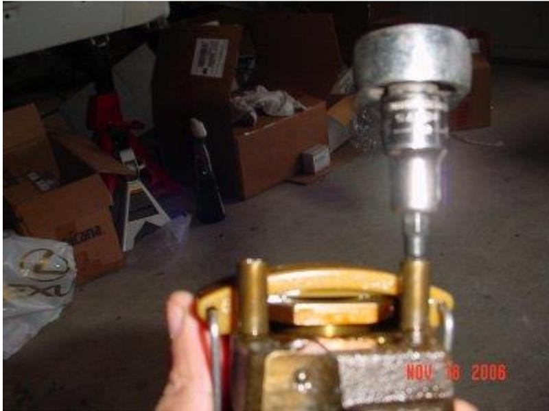
45. Swap the chain on the cams, noting the blue links on both chains, and orienting the new chain just like the old one. The cams should have triangular "arrows" that indicate where the blue chain links should be.
