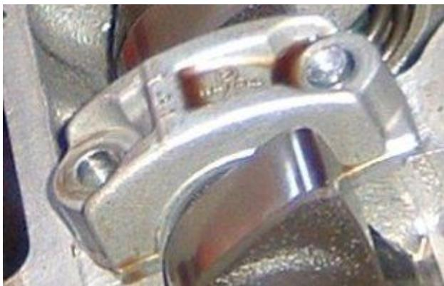
39. As you take each cam carrier (bearing cap) off, be sure to lay them out properly so you can put each one in the same spot it came from, the same way it was.
