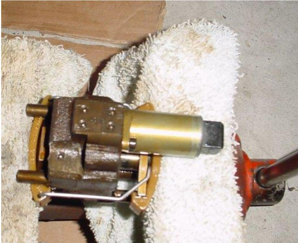
Note: I have done this without a clamp as well (just bare hands). My brother held the cams in the air, and I squeezed the VarioCam into the chain. The cams must be in the air, not laid on a table, whichever way you do it!
