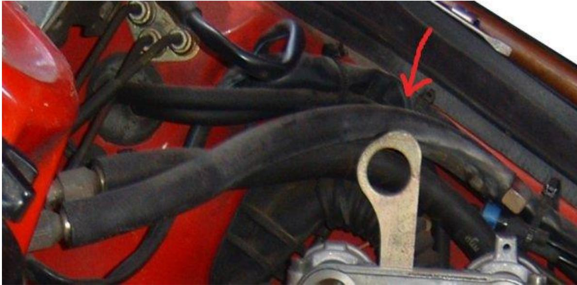
32. Unplug the VarioCam wire from the head and put it somewhere out of the way. You can tuck it under something; I used a zip-tie to hold it to the cruise control cable, over the intake.
