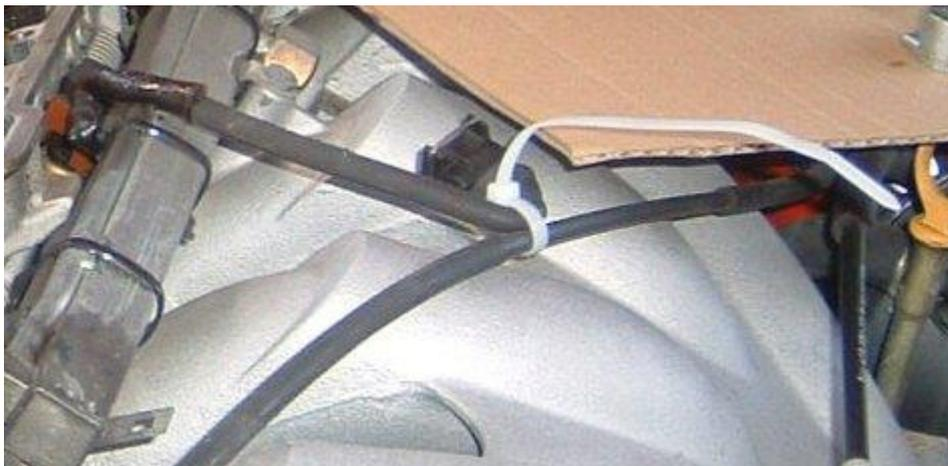
Note, in the above picture, I have disconnected the cruise control cable and have swung it away from the valve cover. Actually, it's easier to just leave the cruise control cable connected.
