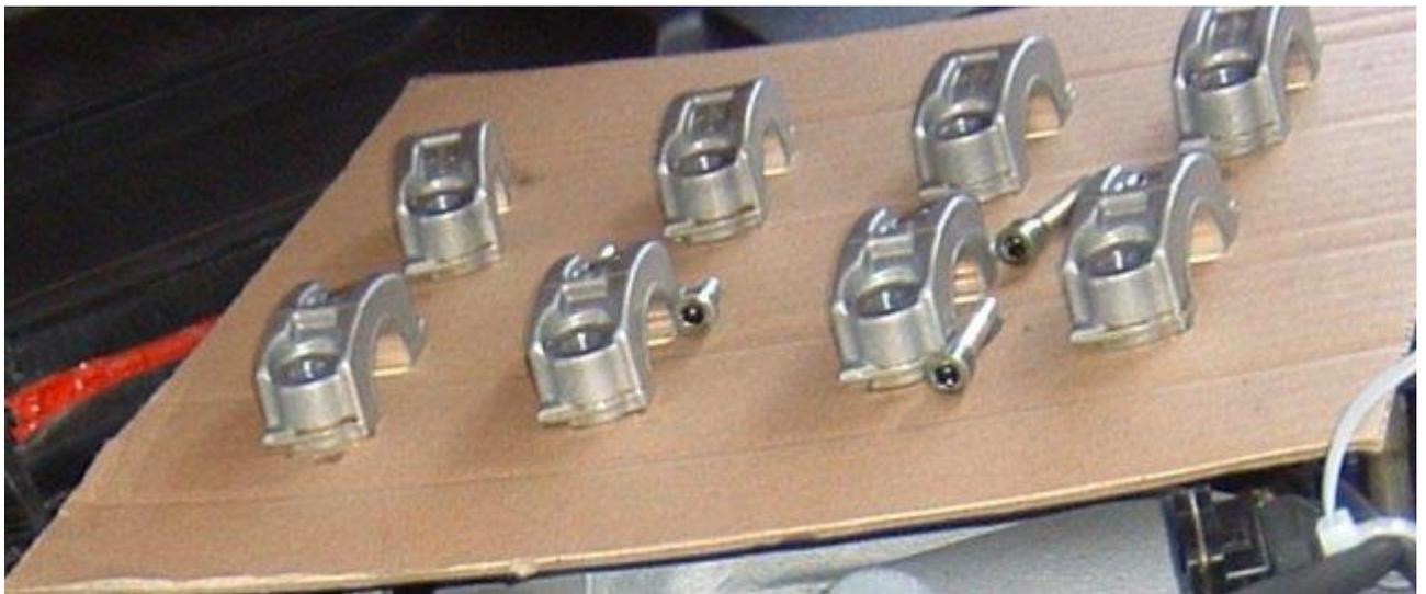
Note: bearing caps are machined with the head they come on, so make sure if you have multiple heads or cam carriers, DO NOT mix them. The trick to telling if they are matching is to look in the middle of the head on the exhaust side by the studs. There is a stamp with the matching number.
