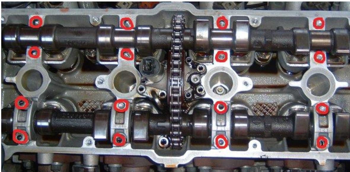
The front 4 go through one solid piece. The other 16 are in pairs, holding the cam carriers down.
