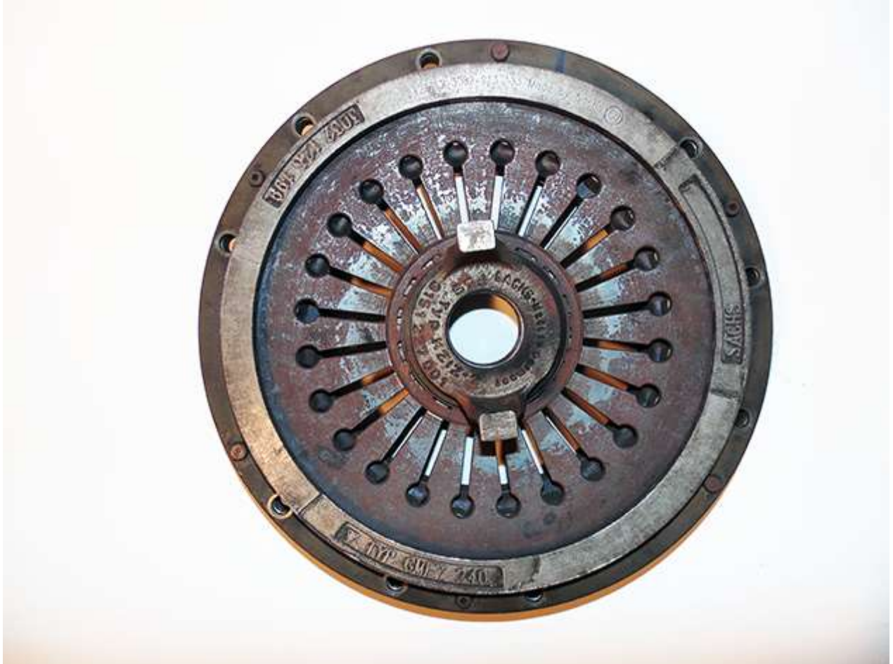
The old "blue-striped" pressure plate 3082-213-133 included in the Sachs clutch kit for the 968.
