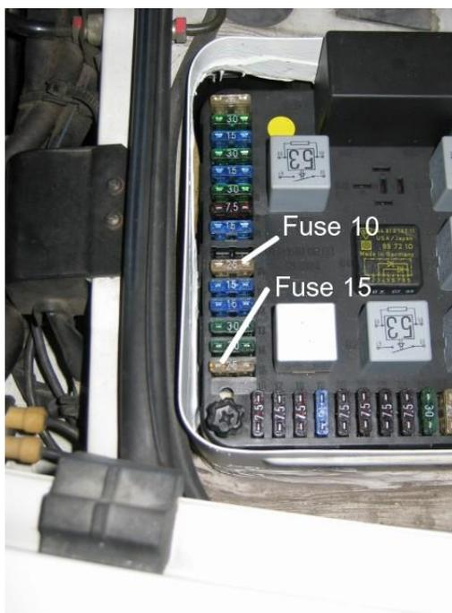
2) **Remove the fan relay**, G10 (the big one), and look at its socket on the relay panel. It will look like this picture. Make a drawing of the socket and identify each connection blade hole on this drawing with its connector name as found on the socket, namely TF, M1, etc. These names are also on the bottom
