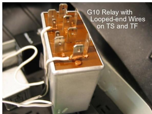
making sure no bare wire comes in contact with the metal can or
