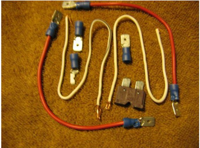
The remaining three will serve as probe-blades, which you will touch with the actual probes of your meter. Two will be used in the wide relay socket holes. Cut the third and last blade in half with a diag. cutter, then cut off one of the halves and file the cut edges. This will be for the narrow relay socket holes. Finally, cut out the fuse wire on one of the cheap fuses; this "defuse" will serve as a probe for the fuse socket.
