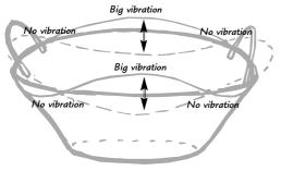
3. The most important vibrations produced are up and down (transverse) vibrations of the metal of the bowl. They travel from the handles round the bowl in both directions. Why both? There is no way of disturbing one bit of the bowl (where the handle is fixed) and making only the metal on one side vibrate!
