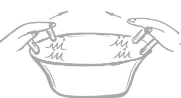
4. The bowl can vibrate in all kinds of ways, but the vibrations that are large and tend to persist are called **standing waves**. They are formed by the vibration of the handle being in step with the vibration that has been round the bowl once and is just passing the base of the handle again! In this way, the energy you put into rubbing the handle ends up in vibrations of one frequency only. This is called "resonance" - the bowl is "resounding" to the vibrations you are providing.
