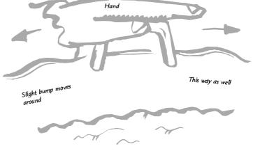
**5.** So standing waves are formed by waves going in opposite directions round the bowl and always being **in step** in some positions. At these positions (called the antinodes) the vibrations get very large. There are also positions where the two oppositely directed waves are always **out of step**, so they cancel out and produce no vibration at that point. If someone touches the bowl at these points (called the nodes), it doesn't stop the bowl from vibrating.
