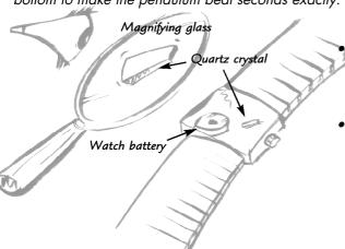
These days, the vibrations of tiny quartz crystals are used instead to keep accurate time.
