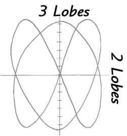
5. As the pendulums swing, they lose energy and so they swing less and less. This makes the patterns drawn by the pen get smaller and smaller, and fills in the gap that would otherwise be in the middle of the pattern.
