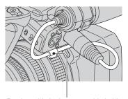
Put the cable in the outer cable holder.
