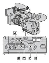
You can adjust and fix the white balance according to the lighting conditions of recording environment. You can store white balance values in memory A (♠ A) and memory B (♠ B), respectively. Unless a white balance is readjusted, values will remain even after the power has been turned off.
