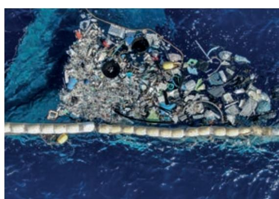
↙ The organisation's system traps debris using a 'skirt' hanging from a buoyancy barrier
