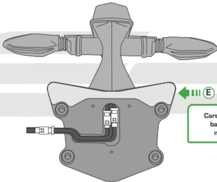
Carefully peel off yellow backing paper from neoprene gasket
