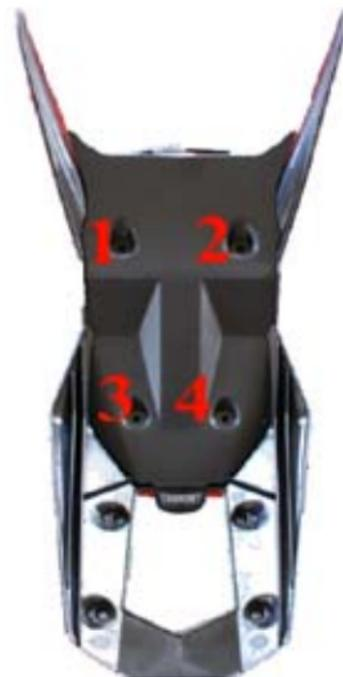
7. Assemble cover plate to the main bracket (see picture below). Feed the indicator wires through the slot before securing the bracket into position using 2 x M4 x 10mm countersunk screws.
