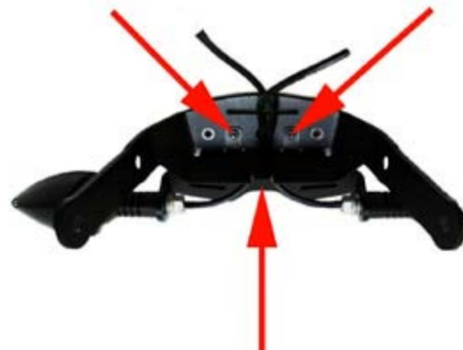
8. Assemble the new DRC light onto the tail tidy using M5 nuts and washers. (See picture below).
