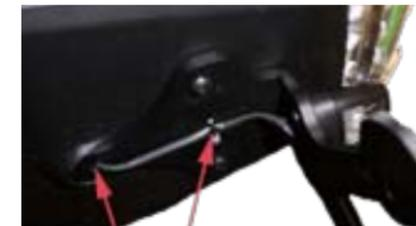
Locate wire and secure with cable tie before assembling to bike
