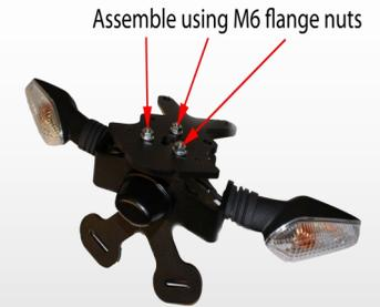
6. Attach turn signals to bracket B using bolts G and crush tubes F.
