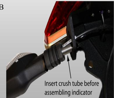
7. Connect turn signals, number plate light to small wiring loom.
