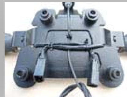
Fig 2. Cable tie the wires as neatly as possible within the milled out area in the upper face of the tail tidy.
