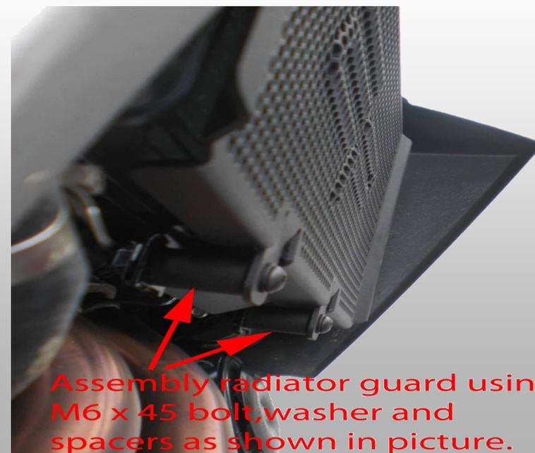
Assembly radiator guard using M6 x 45 bolt, washer and spacers as shown in picture.
