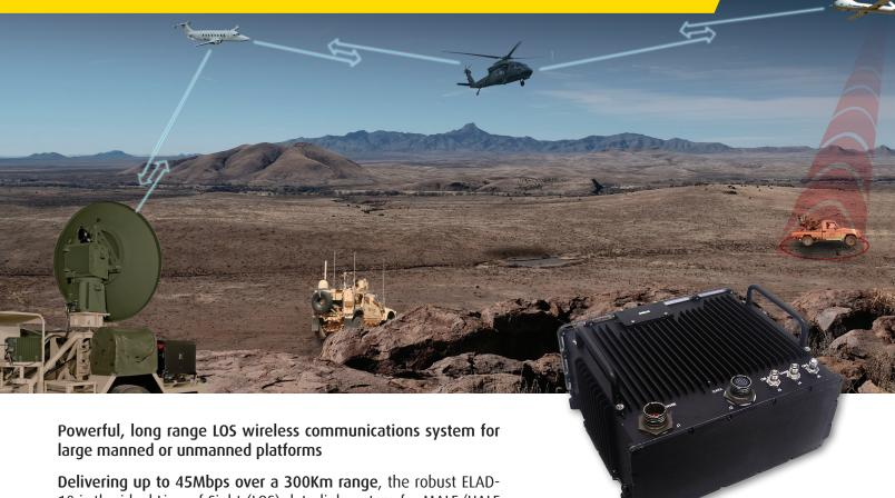
**Delivering up to 45Mbps over a 300Km range**, the robust ELAD-10 is the ideal Line-of-Sight (LOS) data-link system for MALE/HALE UAVs, USVs, mission helicopters, manned mission aircrafts and other long range platforms.
