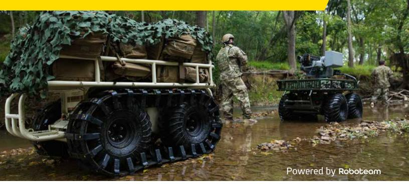
The PROBOT (Professional Robot) platform is designed from the ground up as an autonomous, robust, lightweight tactical support vehicle with high mobility and all-terrain maneuverability in urban and rural environments. Featuring a common all-electric chassis with a very low thermal and acoustic signature, PROBOT can carry heavy payloads and integrate in logistics, medevac, CBRNE, ISR and special operations.
