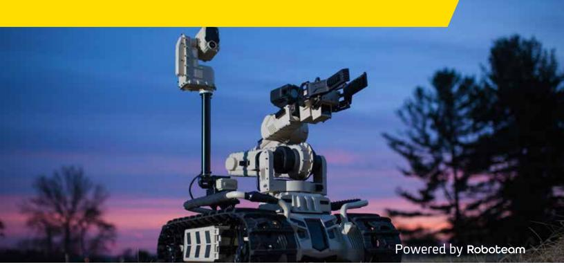
The Transportable Interoperable Ground Robot (TIGR) is a medium-sized, two-person portable unmanned ground vehicle (UGV). The highly mobile, all-weather system is capable of operation in any terrain.
