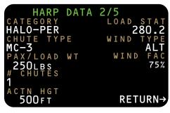
Airdrop Data Page 2 displays information for the selected type of airdrop including chute data, load parameters, and wind considerations.
