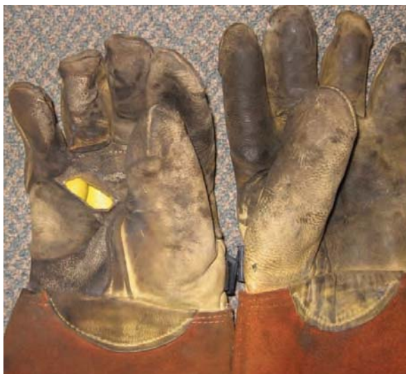
Examples of a fire-resistant shirt (5-6cal/sq cm) and gloves worn by a person burned in a secondary fault, while hooking up some 120/208V leads to a pad mounted transformer. The man came out of the accident with just second degree burns to his arm
