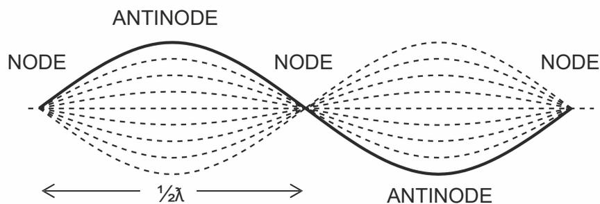
By adjusting the tension and/or vibrating length of a string, notes of higher and lower pitch can be produced. The fixed 500mm (50cm) scales allow for accurate positioning of the movable bridges supplied.
