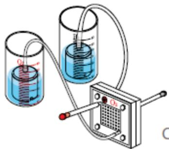
6. The electrolyzer can now be placed onto the module plate and be connected to it using the respective cables (red for O<sub>2</sub>, black for H<sub>2</sub>).
