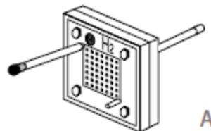
2. The syringe must be filled with distilled water and another short piece of tube should be fitted to it. The other end of the tube must be connected to the upper port on the O<sub>2</sub>-side (red port) (see B).
