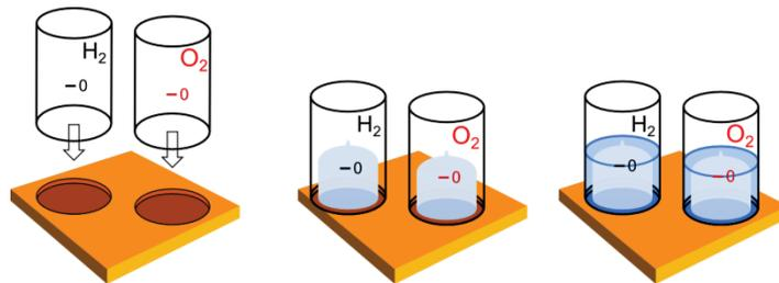
4. Each gas storage tank should be pinned onto the ring mount at the bottom of each water barrel, so that the grooves on the bottom of the gas tanks are aligned with the grooves of the ring mounts. Excess water can be removed using the syringe.
