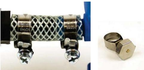
The hose clamps fix and seal the hoses on the turbine casing. They are permanently mounted. The hose for the outflow is hold by a hose clamp with roary knob. When beginning the experiments, this clamp should be used to to turn the hose facing downwards.
