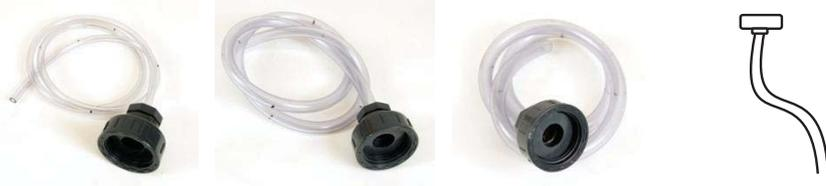
Each flow set consist of a 1m long hose and a connecting piece. The flow sets varaiate in their inside diameter of 4mm, 8mm und 12mm. With the connecting piece the flow set can be screwed to the bottom of the flow box. For marking the hight, every hose have a O ring, which can be pulled to the required place.
