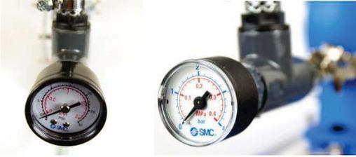
The manometer sets display the pressure the water has flowing into the turbine. The 4 bar manometer is installed on the lower inflow, the 2bar set on the upper inflow.
