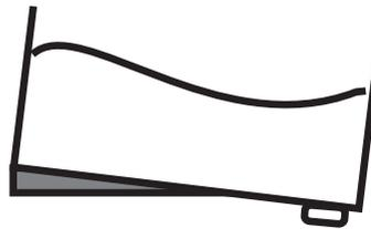
The Flow box has a drain where the flow sets can be screwed onto. It has an inclined bottom so the water can drain continuously.
