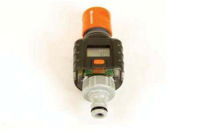
The water volumeter is plugged ontop of the intake connector. It has various programmes, which can be chosen by pressing the orange button. For the following described experiments it is always used the “liters per min” mode.
