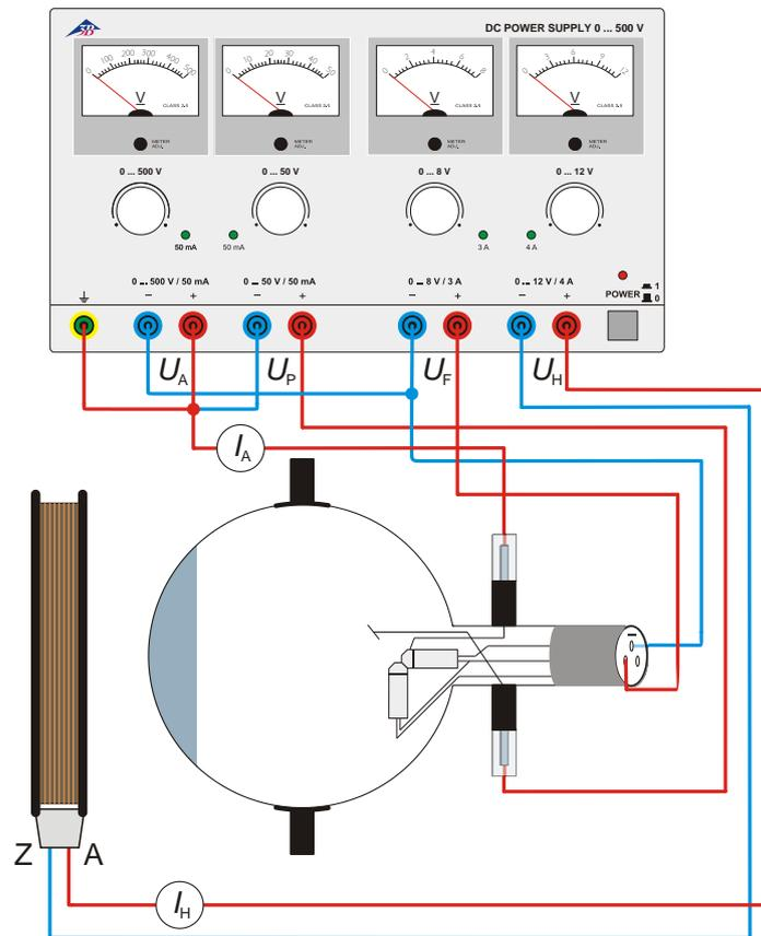
Fig. 6 The effect of an axial magnetic field
