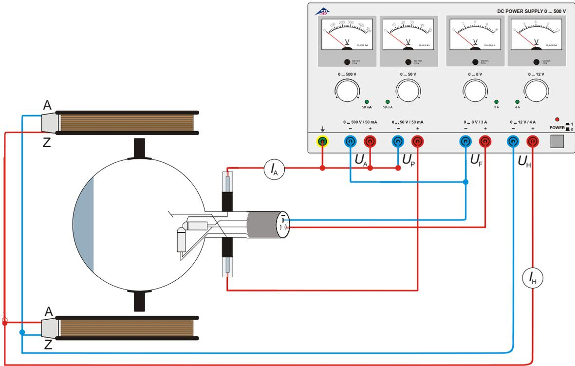
Fig. 5 Determining  $e/m$  using the perpendicular electron gun
