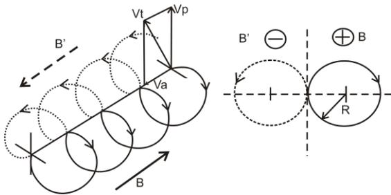
Fig. 3 Helical path of the deflected beam
