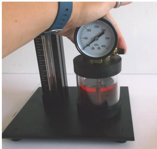
7. Fit the pump nozzle onto the inlet valve correctly
