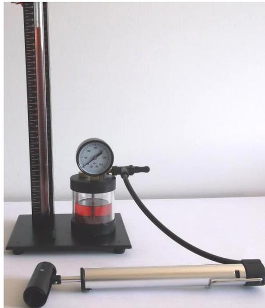
10. Please note, gauge provided, displays the pressure from 100kPa and will require large volume of oil to be pumped into the tube to exceed the pressure of 100kPa
