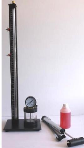
2. Unscrew two valves to equalise the pressure. First screw from reservoir and second one from the top of the column as presented below.
