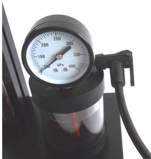
8. Ensure the air valve is open. Turn Anticlockwise to open.
