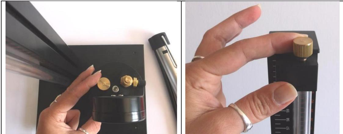
6. Remove the cap on the inlet valve.
