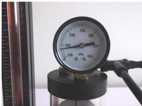
11. Perform the experiment between marked volumes to achieve the best results. Lower mark is recommended at the point where pressure is over 100kPa and the higher point between 15-20 units above.
