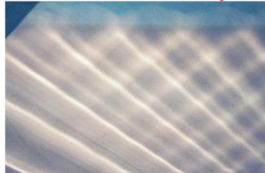
Place a bar in the tank. The ripples will reflect from the bar. If the bar is placed at an angle to the wave front the reflected waves can be seen to obey the law of reflection.
