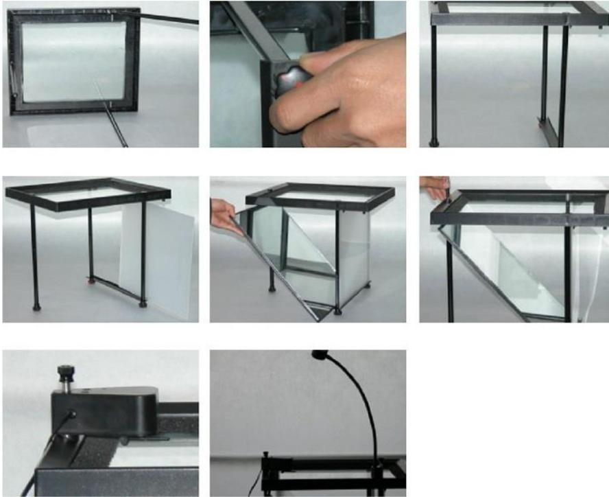
1. Attach the three detachable legs to the ripple tank.
