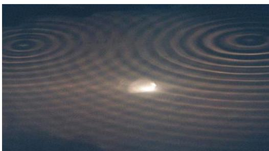
Interference can be produced by using the double dipper. In the diagrams the light areas represent crests of waves, the black areas represent troughs. Notice the grey areas: they are areas of
