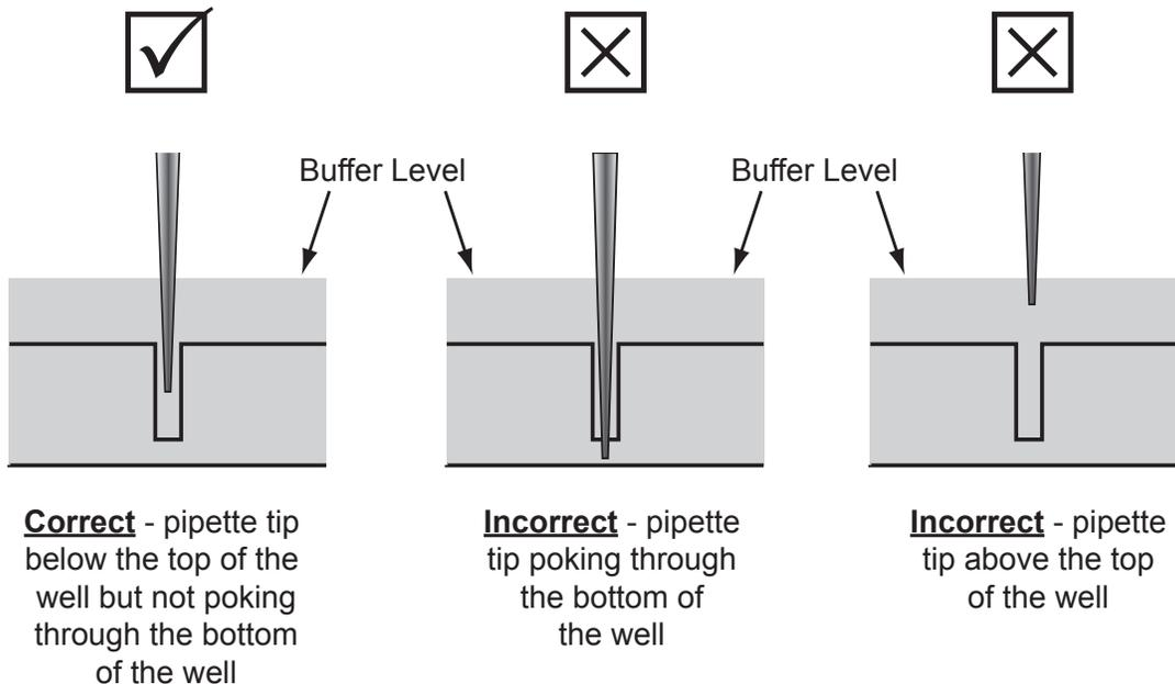
3. Using a micropipette, add 10 $\mu$ l (microliters) of each dye sample to the wells in your agarose gel in the following order:
