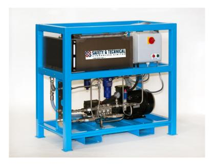
This 30ltr flushing unit has been constructed offering our customer's a simple free standing fixed displacement flushing unit providing 30 litres per minute of flow at a maximum pressure rating of 200 Bar.
