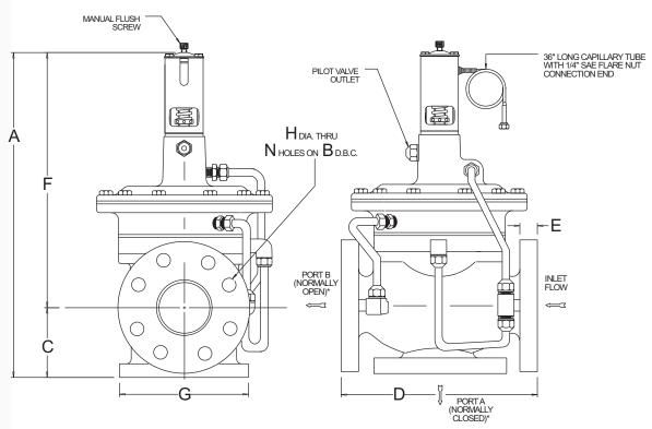
\*NOTE: Normally closed valves open on pressure increase, normally open valves close on pressure increase.
