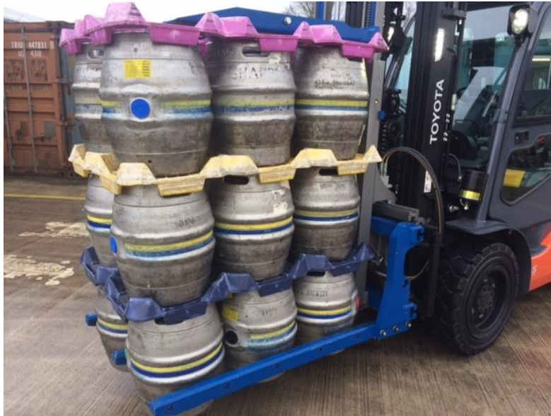
Figure 7: Plastic locator boards holding casks for transport [bandbattachments.com]
