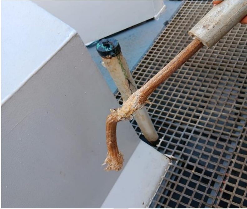
Figure 3-9: Broken towing extension piece
