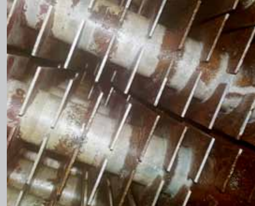
Compacted Ash Removed from Boiler Economisers
