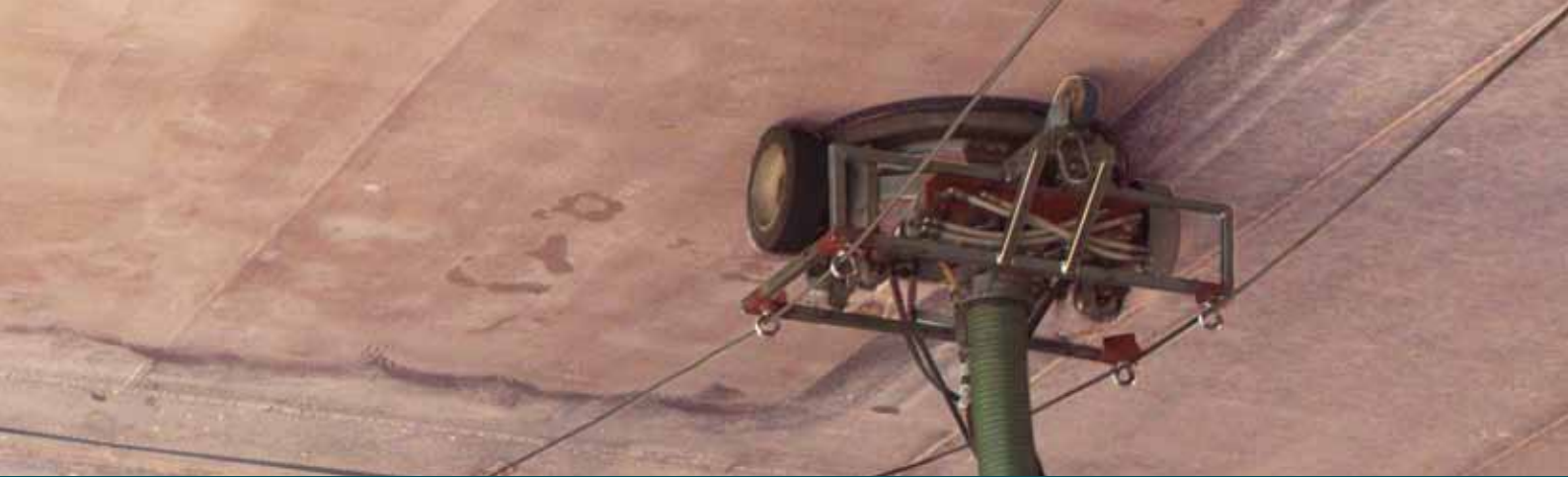
Limpet held inverted by powerful vacuum
