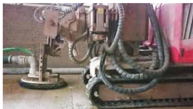
Surface preparation head with brush type vacuum skirt
