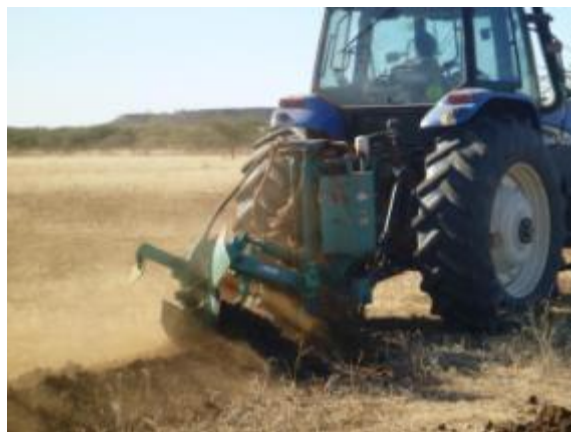
Figure 9: Use of the Delfino plow to break up the compacted soil
