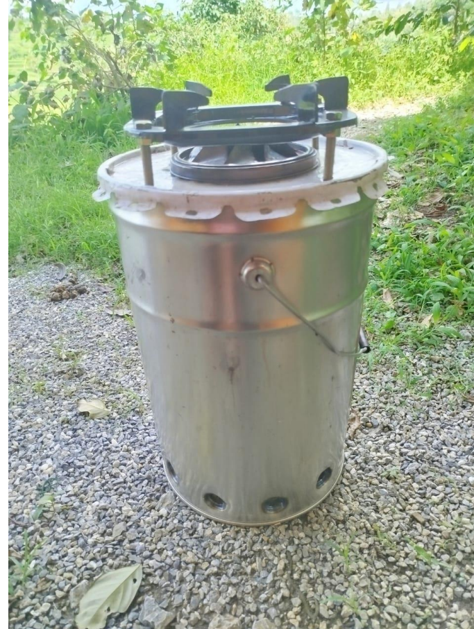
Training by Andalas University staff (Department of Technology) on how to turn household waste into biogas for cooking, using specific biogas burner
