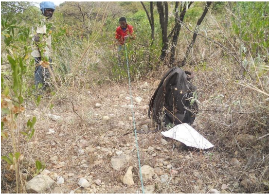
Figure K5: Measurement of soil thickness in augering hole, in a 5x5m compartment.
