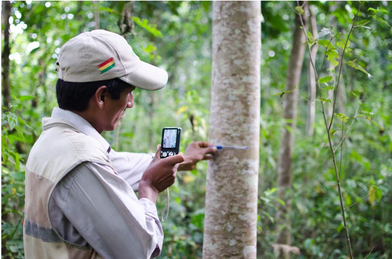
Above: ArBolivia's head of forestry in Rurrenabaque. Moises Andres, takes a photo for quality control. The diameter is measured at "breast height" (dbh), a standard 1.3m above the ground and recorded in the ArBolivia database. Using our new small sawmills this tree is almost good enough for lumber.
