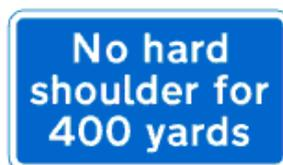
Where links switch between MM-ALR and non MM-ALR then the distance on the 'no hard shoulder for XX miles' sign should be to the start of the hard shoulder for the downstream non MM-ALR link. At the end of the non MM-ALR link a 'no hard shoulder for XX miles' sign shall be included for the downstream MM-ALR link. A 'no hard shoulder for XX miles' sign is not required intra-junction at non-TJR junctions.
