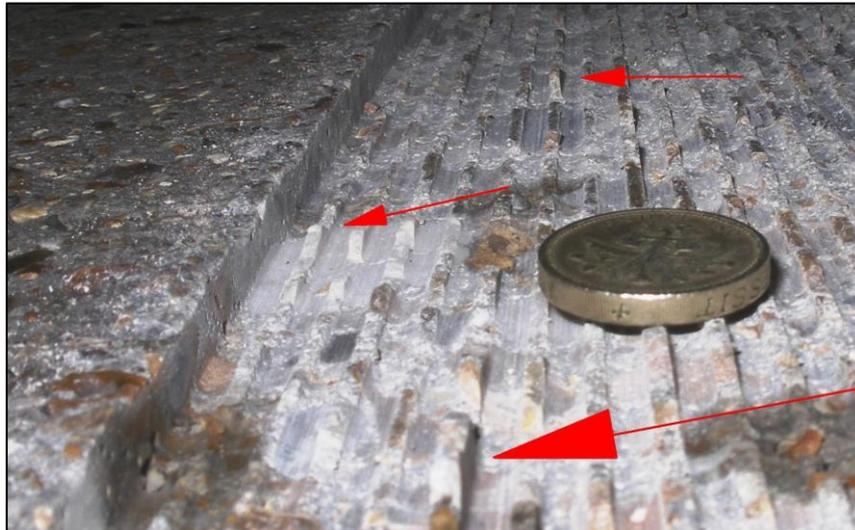
**Figure 2-2 Surface finished achieved with diamond grinding technique**
