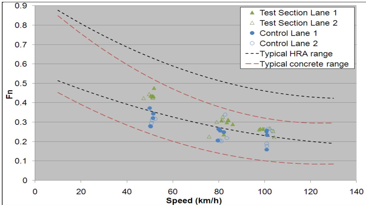
**Figure 3-7 Locked-wheel friction northbound after 7 months**
