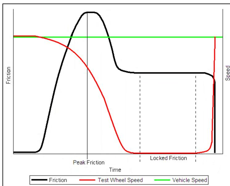
**Figure 3-4 Idealised graph of an average wet PFT skid test**
