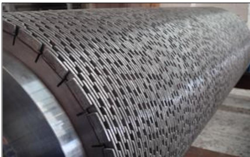
**Figure 2-1 Profiled diamond grinding drum**
