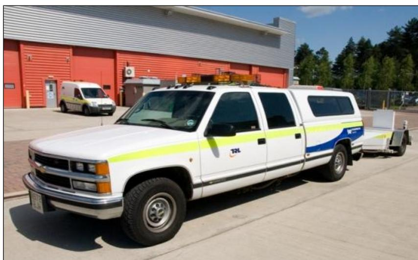
**Figure 3-3 Pavement Friction Tester**
