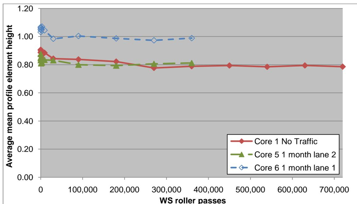
**Figure 4-5 – Mean profile element height absolute values**
