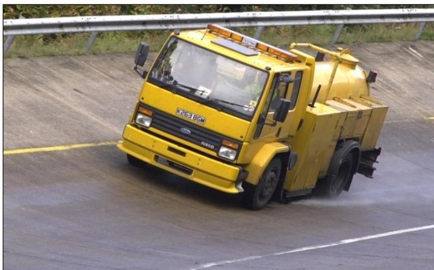
**Figure 3-1 SCRIM testing a section of the TRL test track**
