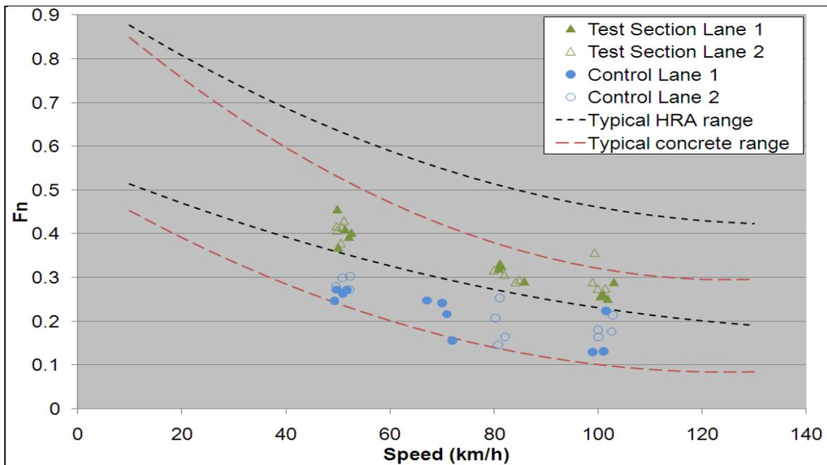
**Figure 3-8 Locked-wheel friction southbound after 7 months**
