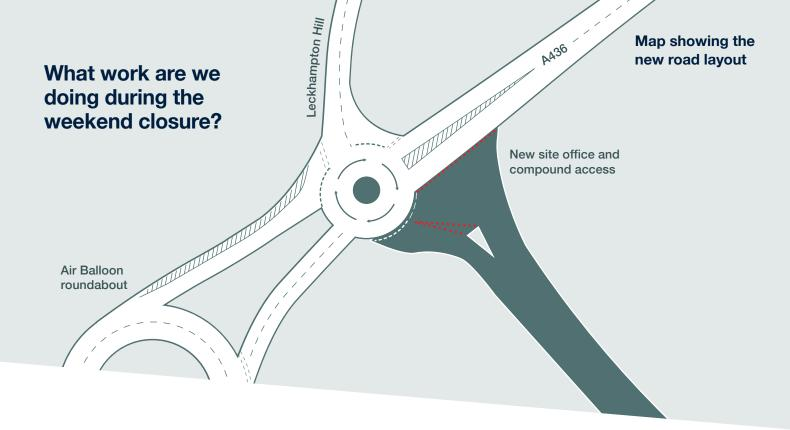
During this work we'll remove existing traffic islands, create a temporary roundabout and install a new site entrance.
