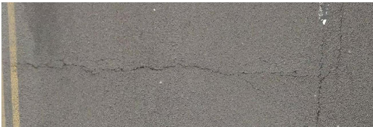
Figure 10: Transverse and Longitudinal Cracks (c)
