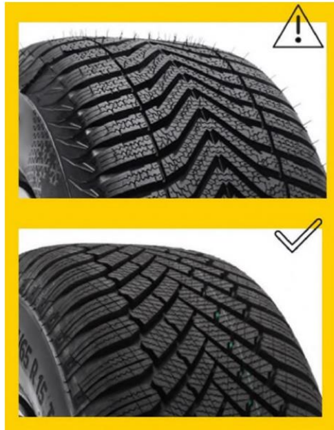
Figure 2-10: Tyre shown with (top) and without (bottom) vent spew threads; Source: [75]
