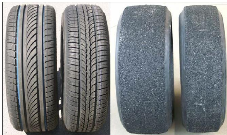
Figure 2-11: Two porous tread tyre prototypes (right) alongside regular tyres (left) used as carcasses for the porous tread; Source: [80]
