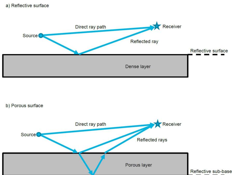
Figure 2.1: Sound Paths over Reflective and Porous Surfaces
