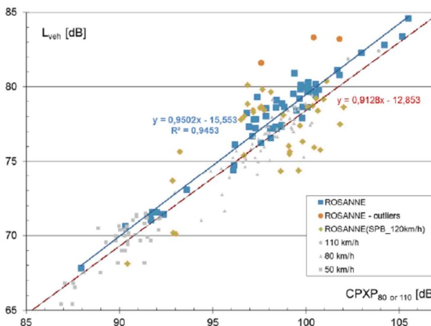
**Figure 5.1: Normalised CPX and SPB Data, for Category 1 Vehicles, Collected from the ROSANNE Project<sup>7</sup>**
