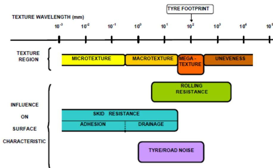
Figure 2.3: Texture Wavelengths and Influence on the Surface Characteristics<sup>1</sup>
