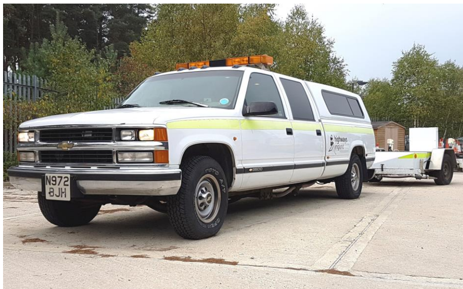
Figure 2-1 The Pavement Friction Tester (PFT)
